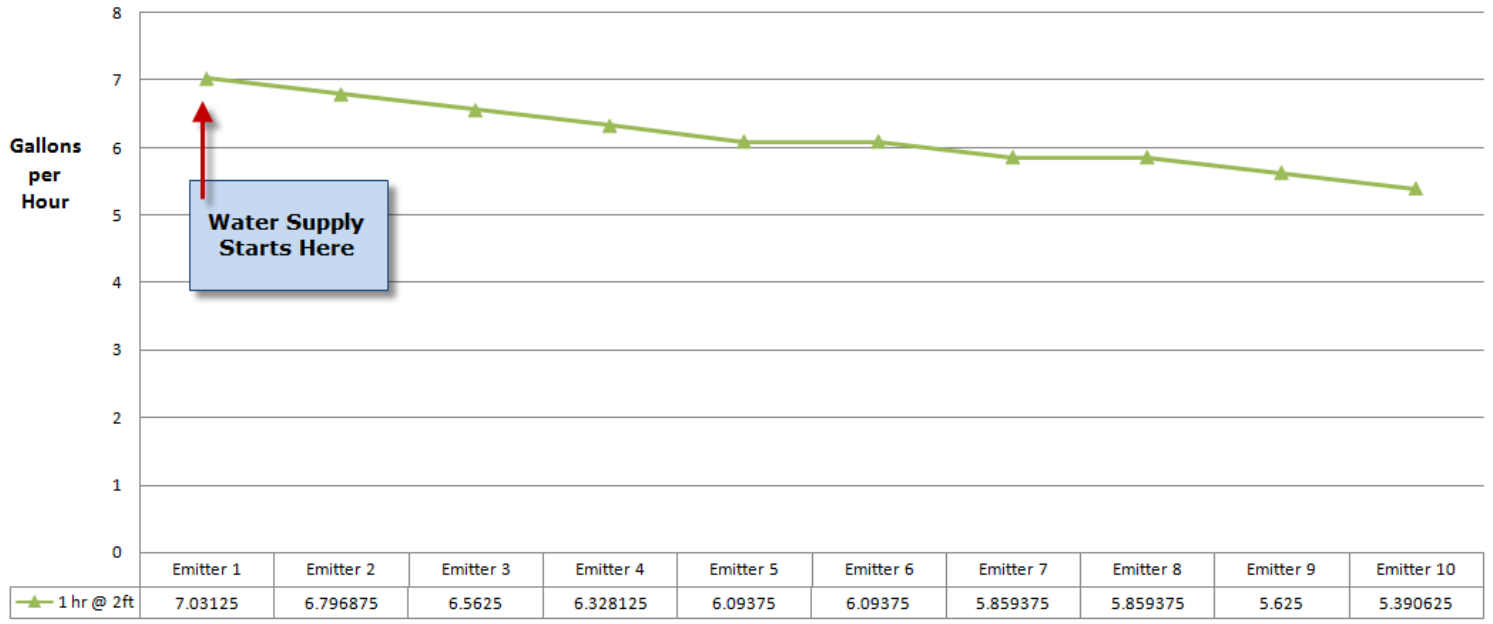
Flow Control Valves (FCV250) --- Rain Barrel @ 2 ft elevation
